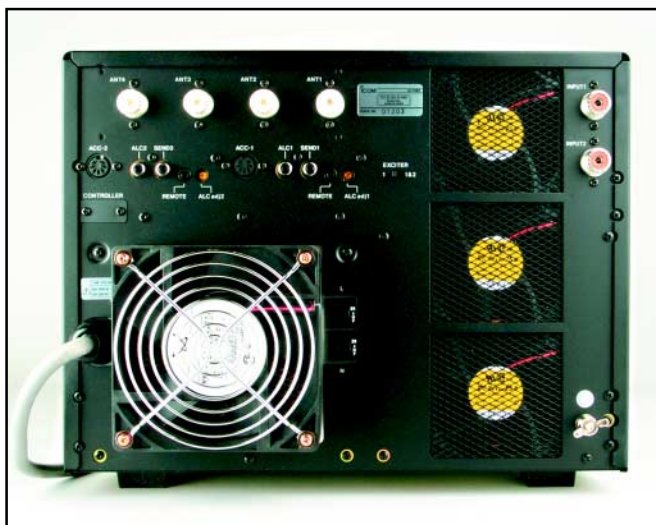
Figure 8—The rear panel of the ICOM IC-PW1 offers input, ALC, switching and control connectors for two separate exciters and outputs for up to 4 antennas.
