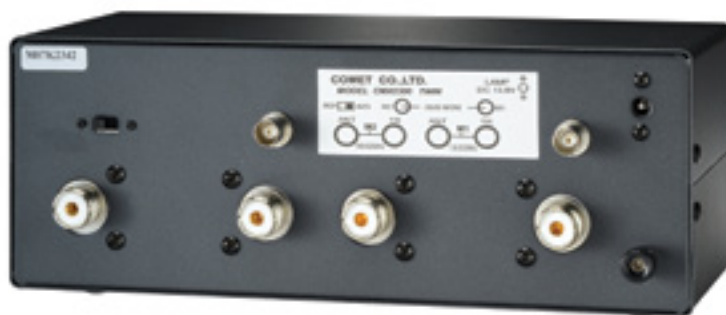
The rear of the CMX-2300. Note the BNC ports for sampling attenuated RF.
